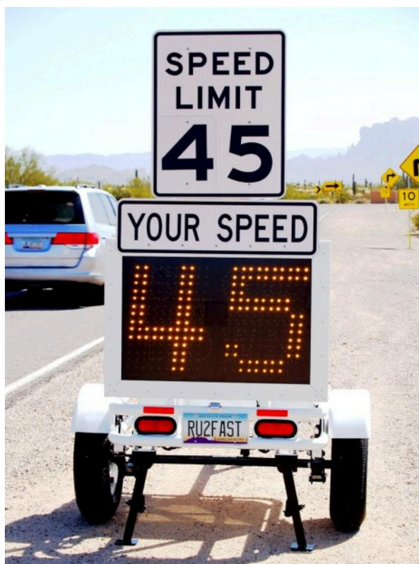
The Fast 820 Radar Speed Display Trailer features a 18" tall full matrix character display for easy viewing and quick driver recognition over 1200 feet down range. When deployed the Fast 820 stands over 8 feet tall. The speed limit sign folds down creating a lower trailer profile for easy transport and storage. Standard features include adjustable high and low blanking speeds, flashing digit violator alert and, traffic management arrows.
