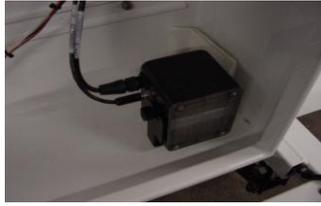
*Figure 5b - Internal Radar Gun swivels both Horizontally & vertically for diverse aiming options*
